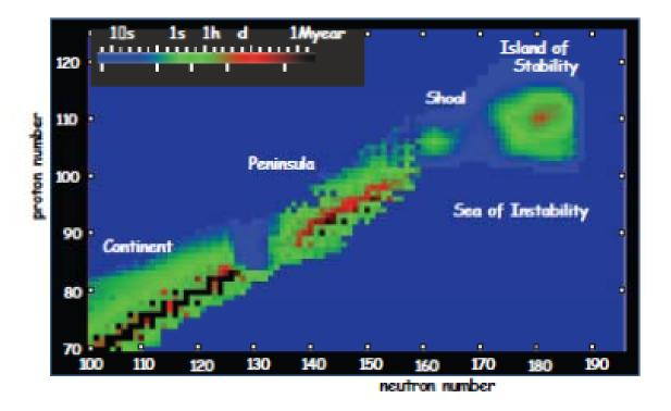
**Fig. 4** A picture clearly evidencing the regions of existence for isotopes with Z > 70 and N > 100. The blue area indicate the "sea of instability" where elements can not exist. The color scale from blue to black displays the increase in life-time (Courtesy by Yu.Ts. Oganessian, reproduced from Oganessian 2019, pag. 06)
